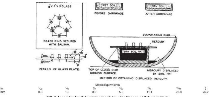
FIG. 1 Apparatus for Determining the Volumetric Change of Subgrade Soils
