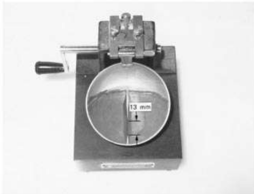
FIG. 7 Soil Pat After Groove Has Closed
