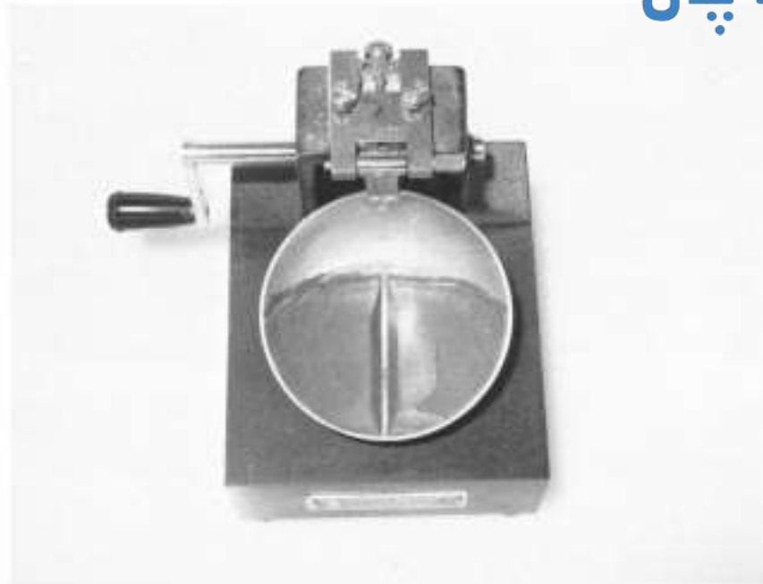
FIG. 6 Grooved Soil Pat in Liquid Limit Device
