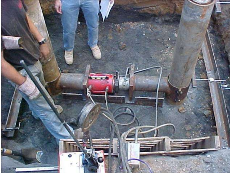
Figure 7-6. Photograph of Lateral Load Test Set-Up (Note: Two micropiles are tested simultaneously).
