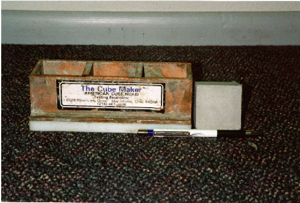
Figure 8-7. Grout Cubes for Compressive Strength Testing.
