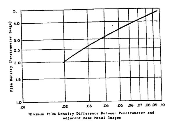
Figure 4. Minimum contrast of radiographs at various film densities.
