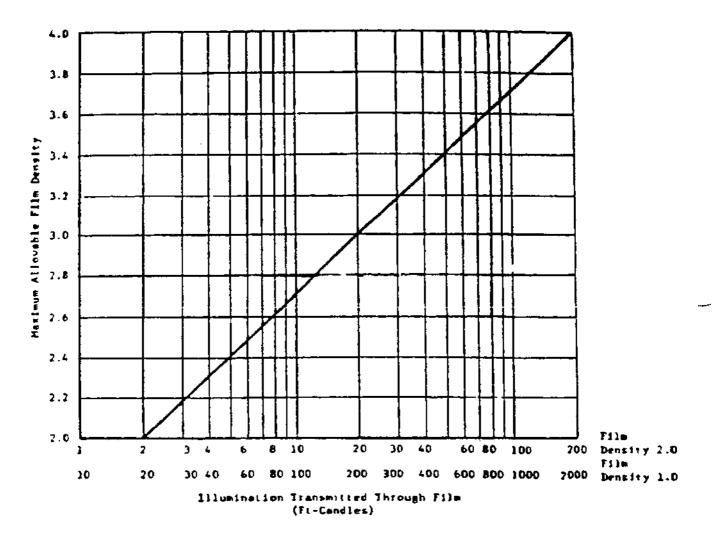
Figure 1. Maximum allowable film density usable with film viewer.
