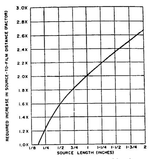
NOTE: To find the source-to-film distance to use with a given source, find the minimum source-to-film distance from Figure 5, and multiply this value by the length-factor from the above curve.
